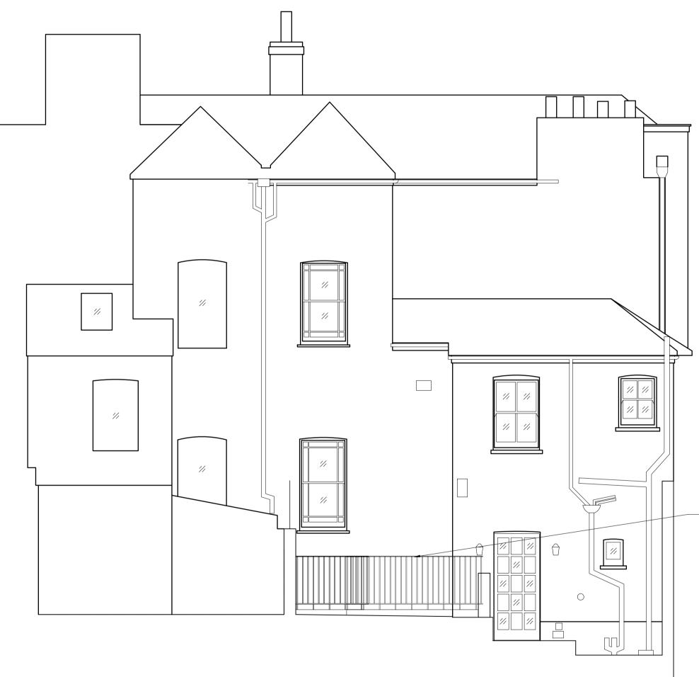
Existing wall copings replaced with more suitable material. Existing handrails replaced with more appropriate design using cast iron
