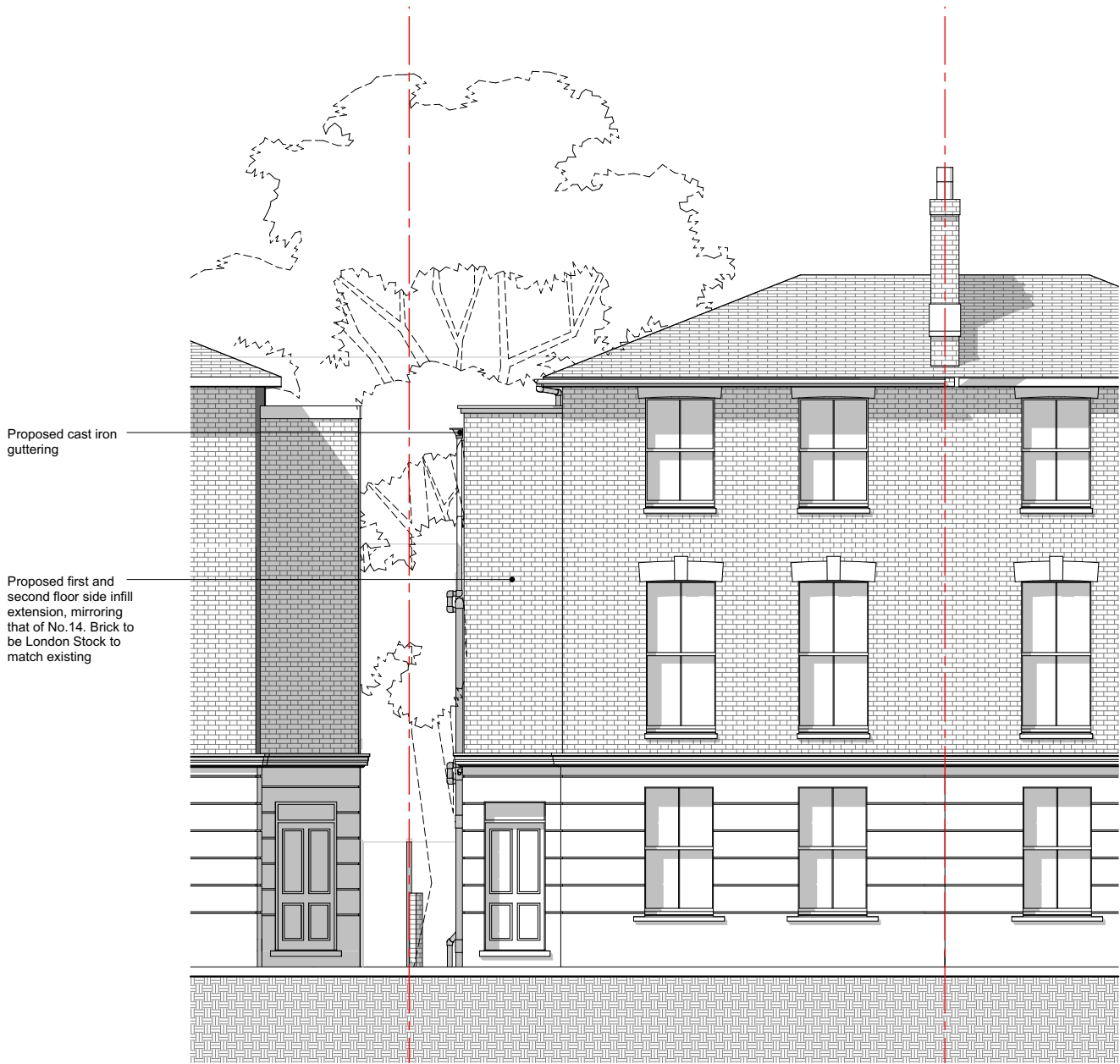
PROPOSED FRONT (EAST) ELEVATION SCALE: 1:100@A3
