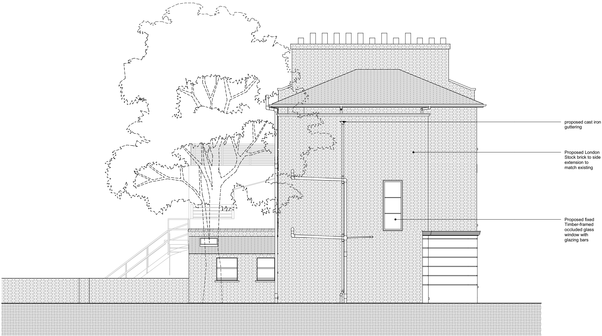
PROPOSED SIDE (SOUTH) ELEVATION SCALE: 1:100@A3
