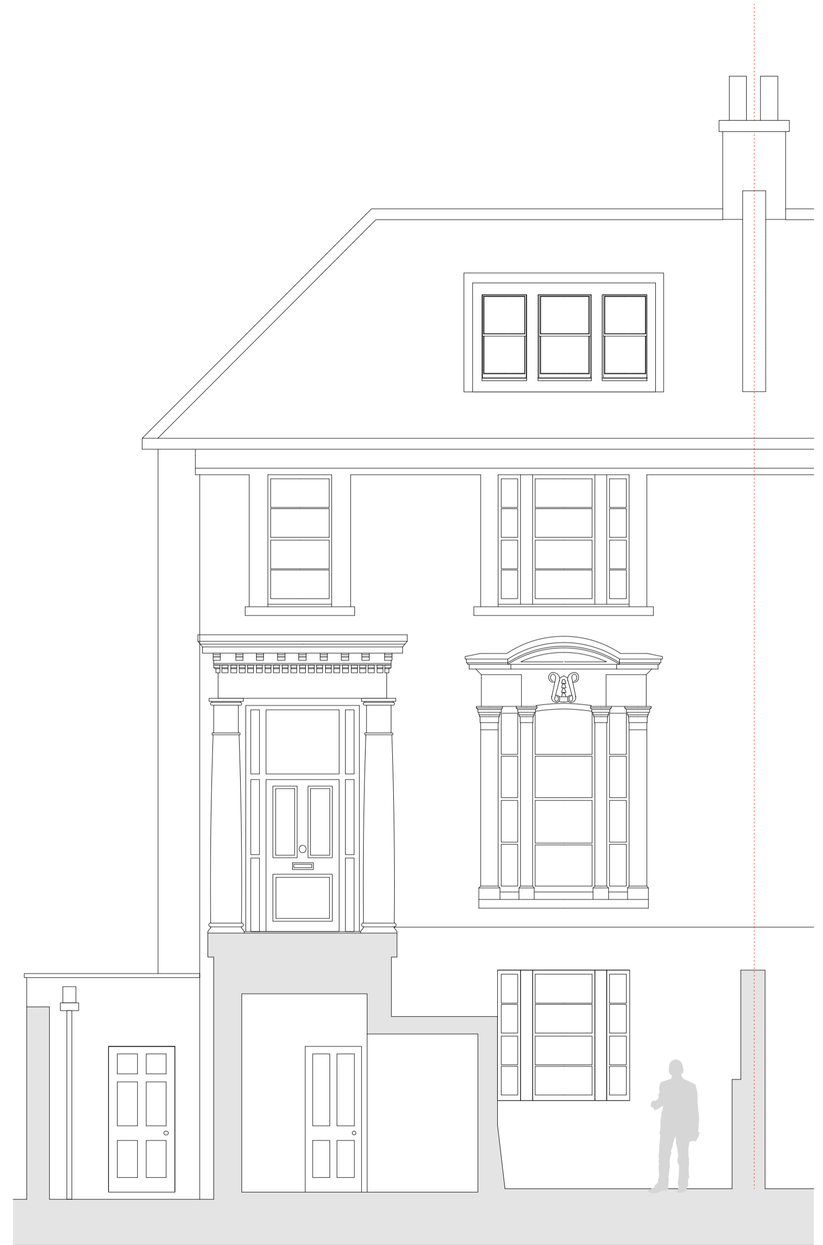
FRONT ELEVATION - SECTION THROUGH LIGHTWELL
