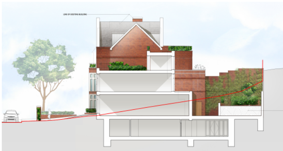
Proposed Section AA with overlay of slope of land from existing section AA (above)
