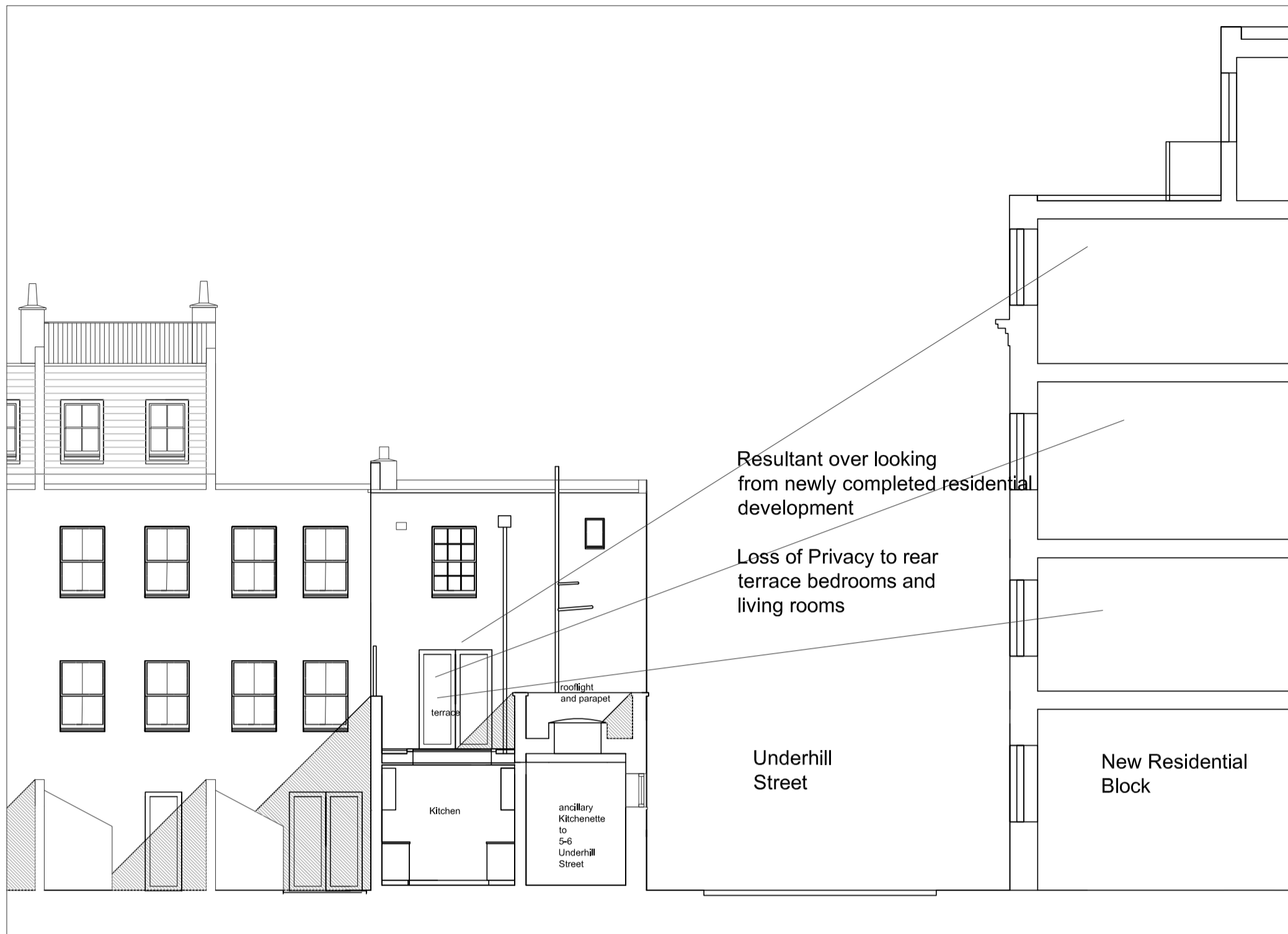
Existing Rear Sectional Elevation in context 1 to 100
