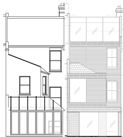
COMPARISON IN SCALE BETWEEN APPROVED EXTENSION AT NO. 2 (LEFT) AND PROPOSED REAR/SIDE INFILL EXTENSION (RIGHT)
