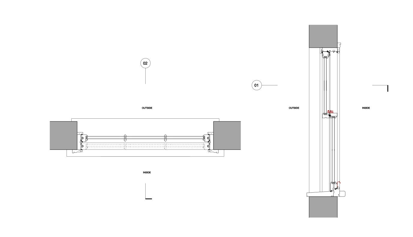
01 SIDE WINDOW TIMBER SASH PLAN PLAN PLAN-SCALE 1:10 @A3
