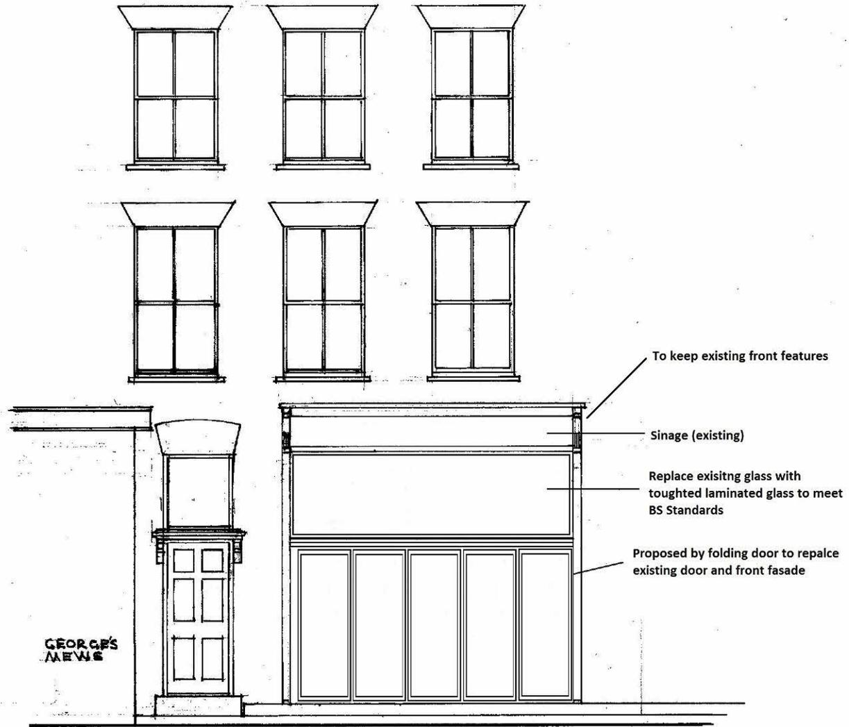
Proposed Front Fasade Elevation
