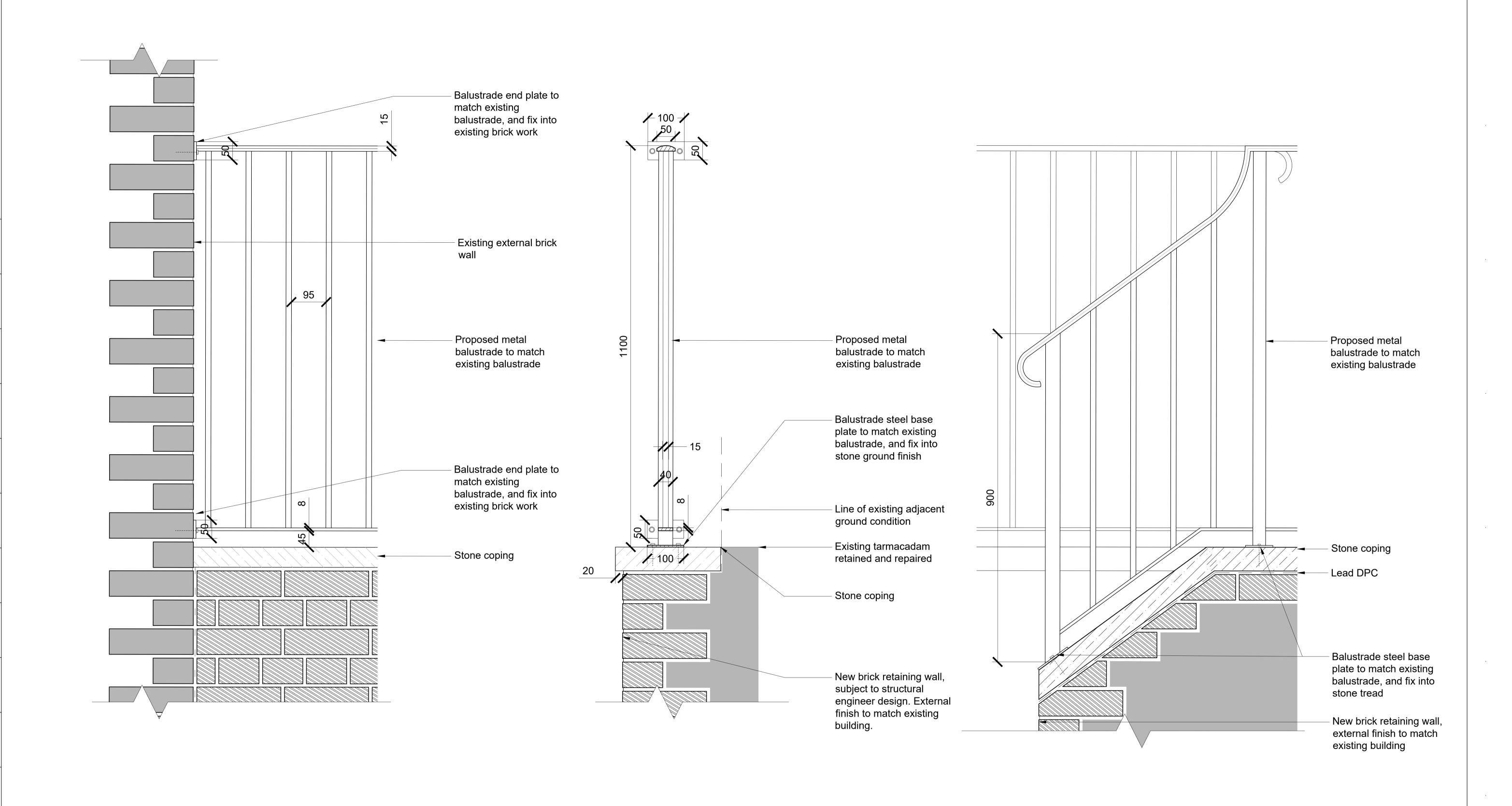
1 - BASEMENT LIGHT WELL DETAIL: BT02 BALUSTRADE TO EXISTING BRICK WALL 2 - BASEMENT LIGHT WELL DETAIL: BT02 BALUSTRADE TO NEW STONE COPING
