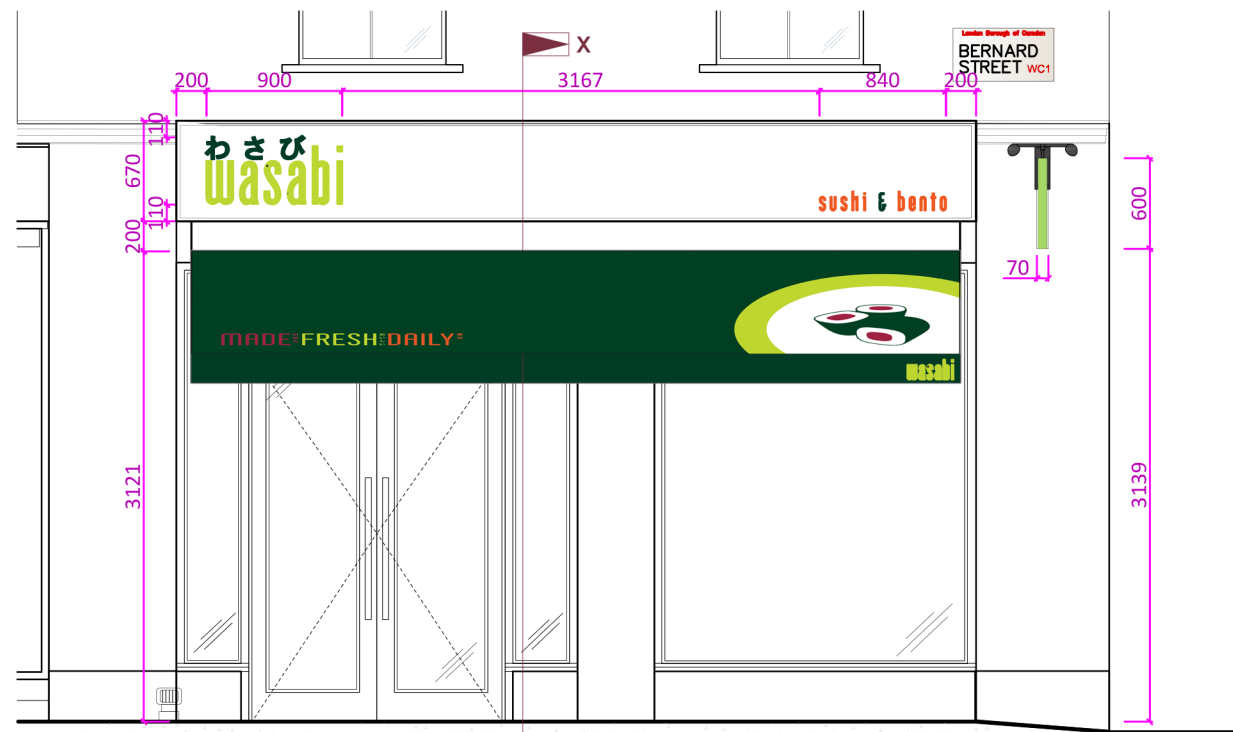
Shopfront Elevation - Awning open Scale 1:50
