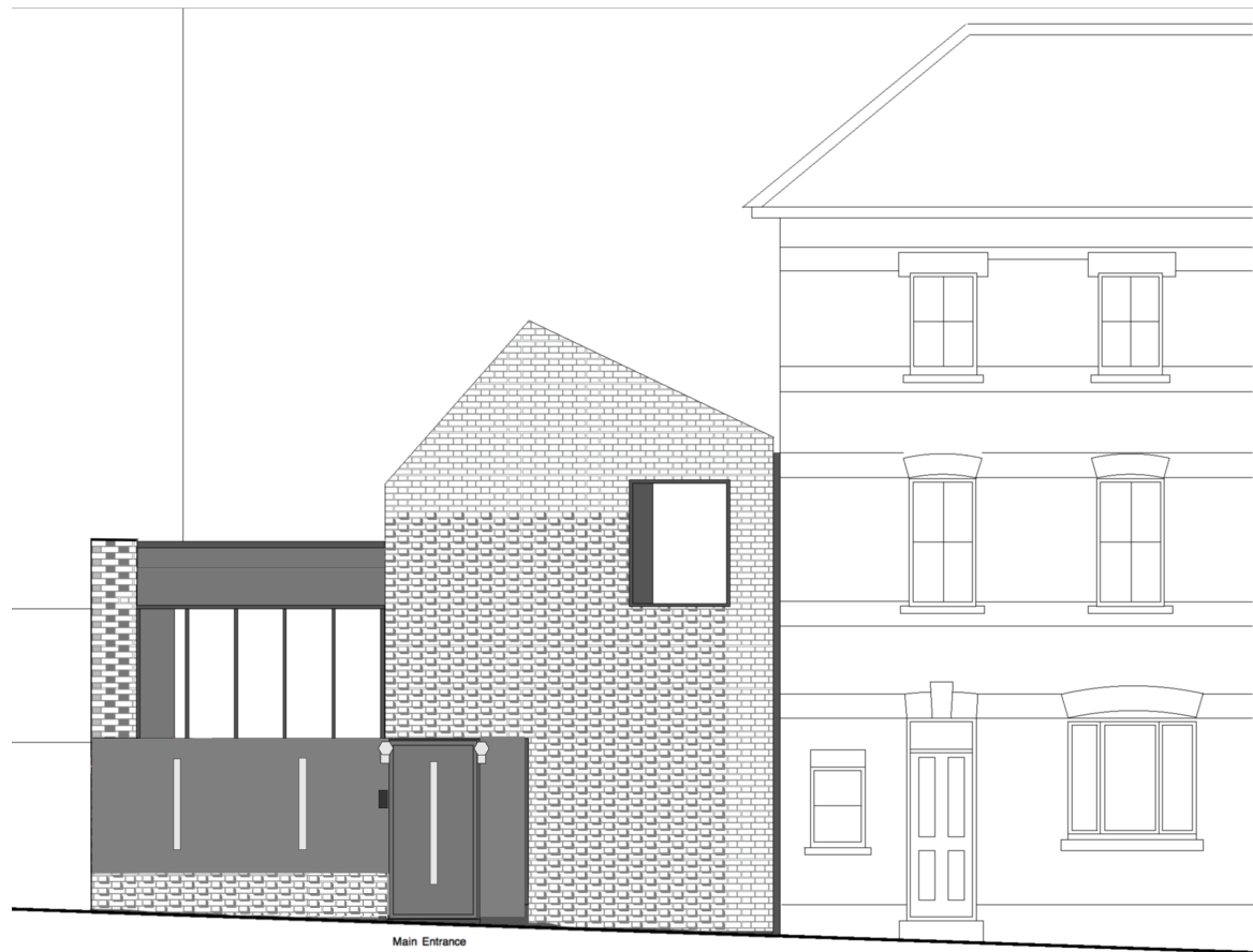
NEW COPPER HAMMERED STEEL PLATE FENCE AND ENTRANCE.
