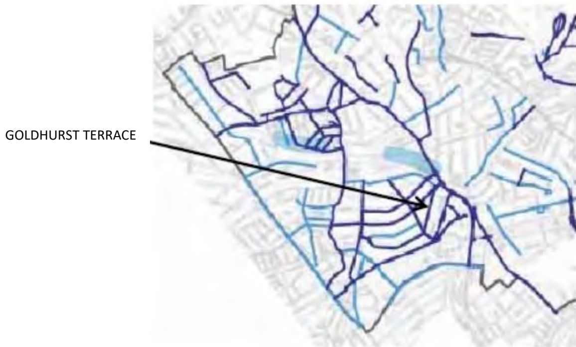
Figure 3. Extract from Figure 15 of the Camden GHHS (Arup, 2010) showing roads which flooded in 1975 (light blue), in 2002 (dark blue), and 'Areas with potential to be at risk of surface water flooding' (wide light blue bands).
