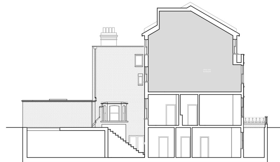
Proposed- Section showing the addition of the basement and the side addition
