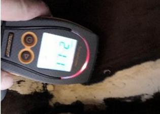
The remaining joists and rear wall plate are highly vulnerable to fungal decay.
