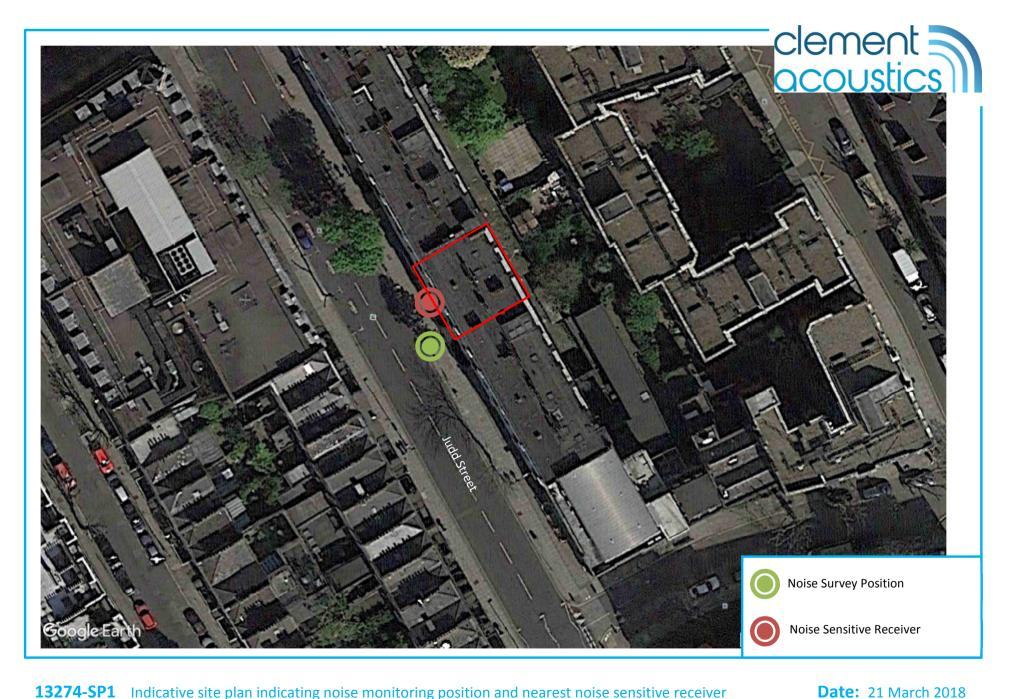
**13274-SP1** Indicative site plan indicating noise monitoring position and nearest noise sensitive receiver
