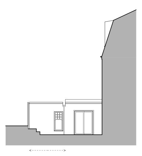
SIDE ELEVATION OF new timber sliding REAR EXTENSION
