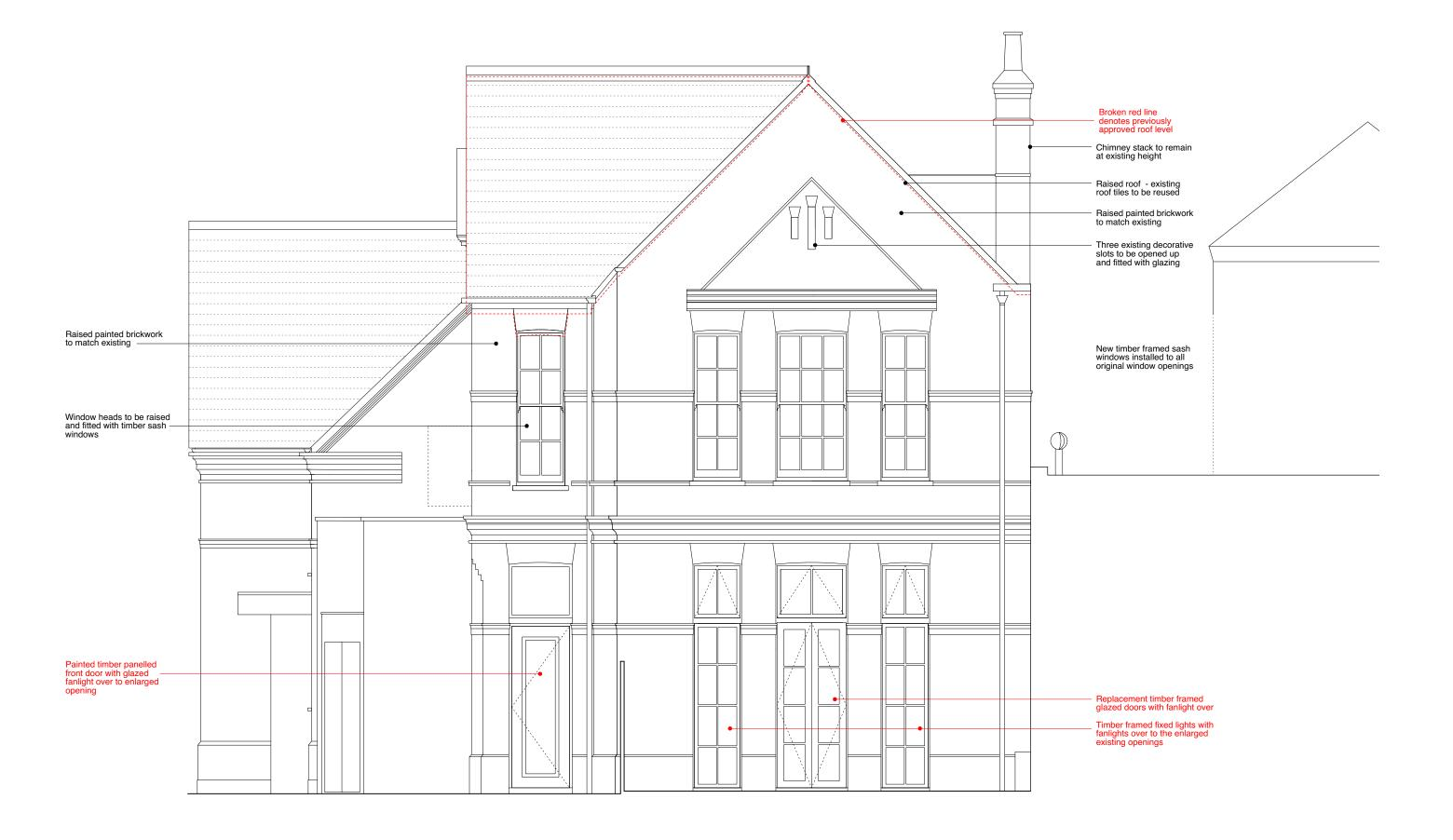
Rev.D 23.02.18: No amendments further to those listed under Rev.C Rev.C 13.02.18: Roof level raised by 2 brick courses (c.150mm); intermediate glazing bars added to the sash windows, fixed lights and doors. Rev.A 22.03.17: Roof finish note added.
