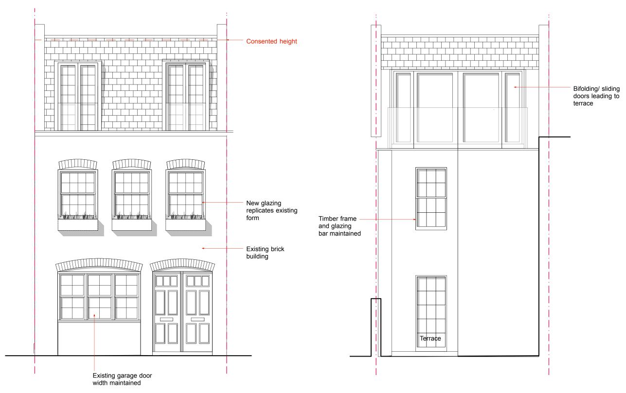
Front Elevation Rear Elevation
