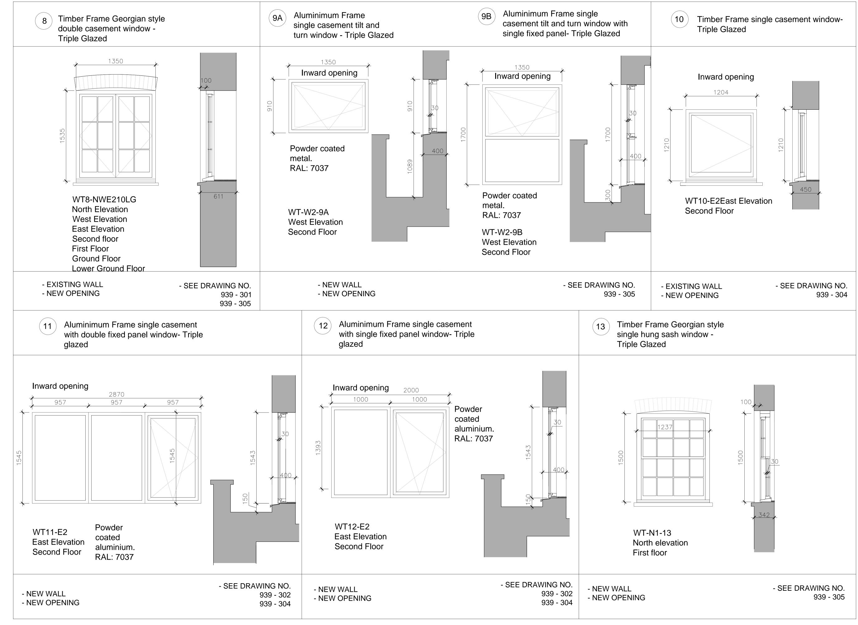
Window Key: The WT is the window type with the window type number. The Next letters stand for where it occurs in the building, for example South elevation first and ground floor would read S01
