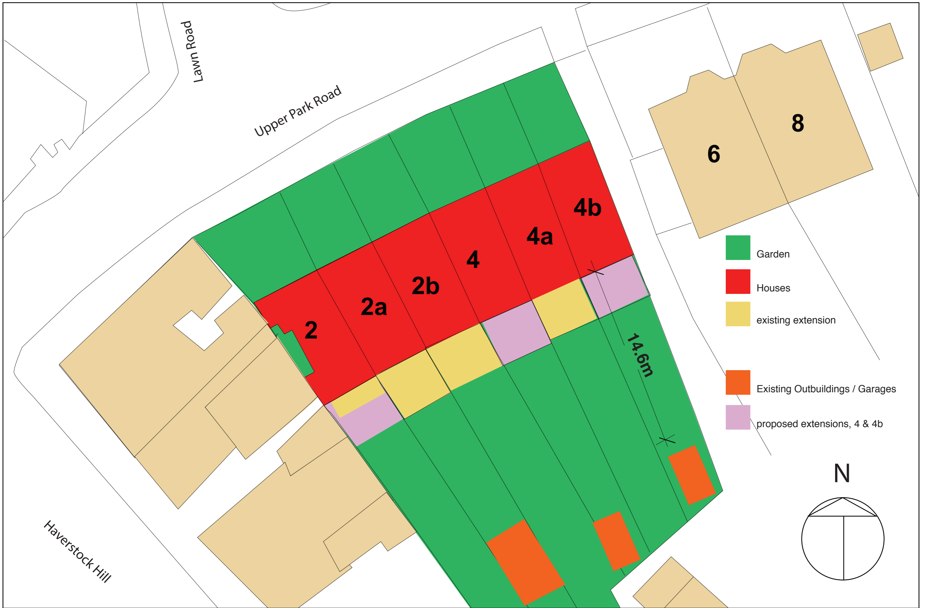
Drawing 002 - Site plan. Scale 1:200
