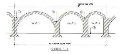
PRIOR TO CONSTRUCTION OF ANY OF THE VAULT ARCH PROTECTION OR SUPPORT. INSPECTION AT LOCATION 1 TO 4 IS REQUIRED. THESE AREAS WILL BE OPENED UP AS ONE OF THE EARLY STAGES OF WORK, AND IT IS INTENDED INSPECTION IS CARRIED OUT AS WORK PROCEEDS AND NOT AS PRE CONSTRUCTION INVESTIGATION WORKS.
