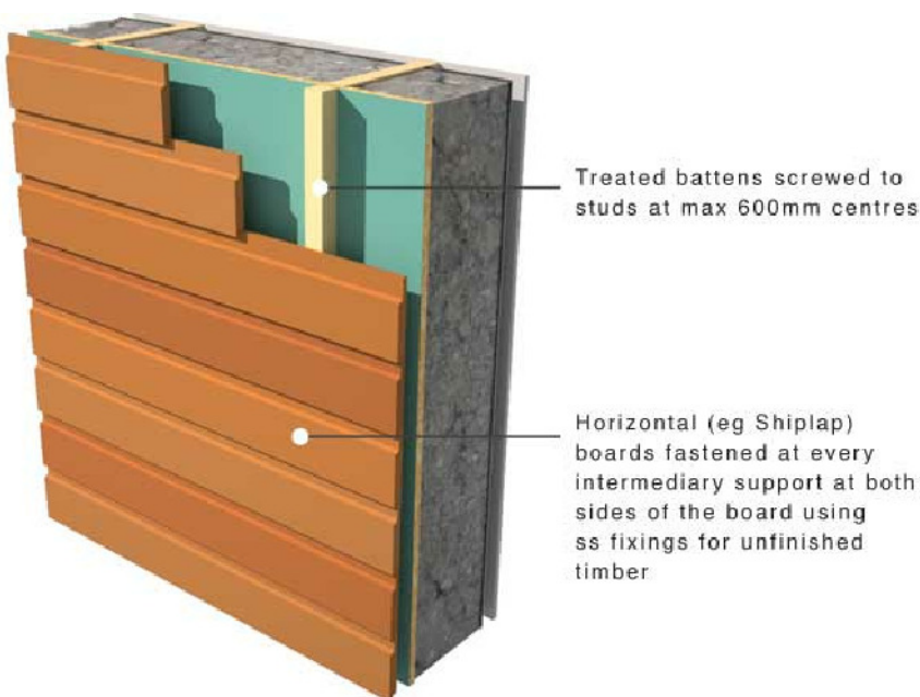
7A TIMBER CLADDING 3D DETAIL
