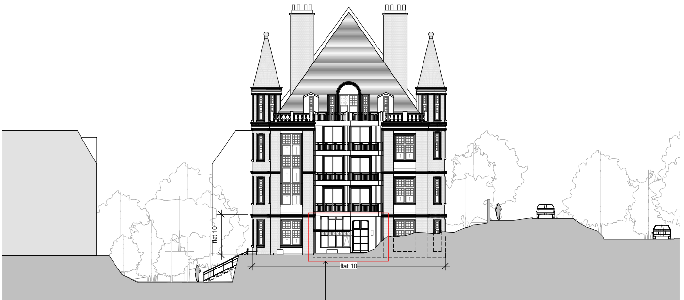
Existing conservatory with wooden frames and clear glass infill
