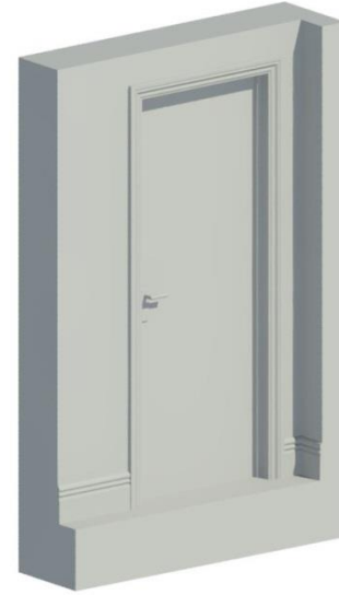
Typical existing moulded architrave doorframe and door
