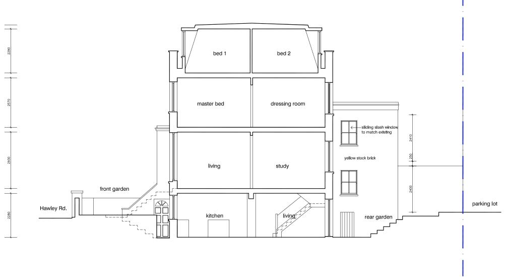
sectional elevation BB as proposed
