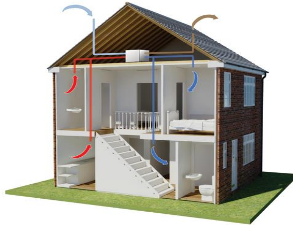
Figure 9: Typical domestic mechanically ventilation with heat recovery (MVHR) system.
