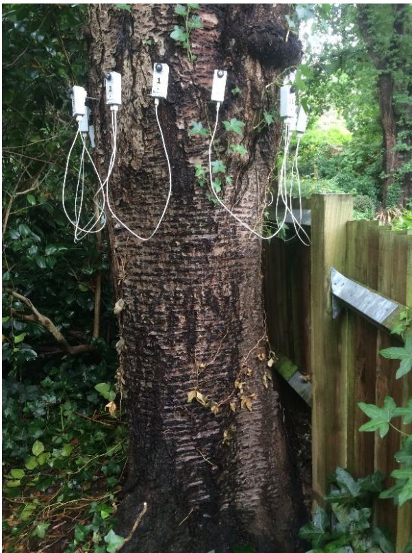
Photo 3: Showing sensors attached to stem at 170cm above ground level, south side
