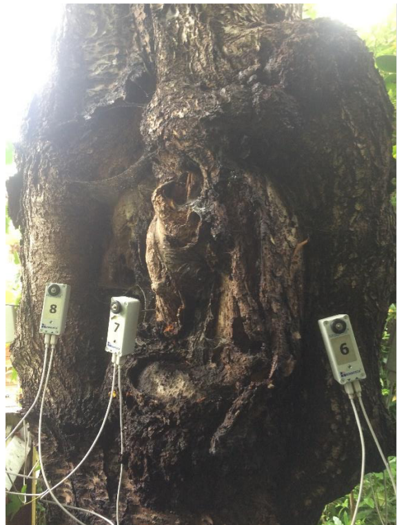
Photo 2: Showing sensors attached to stem at 170cm above ground level in zone of wound.
