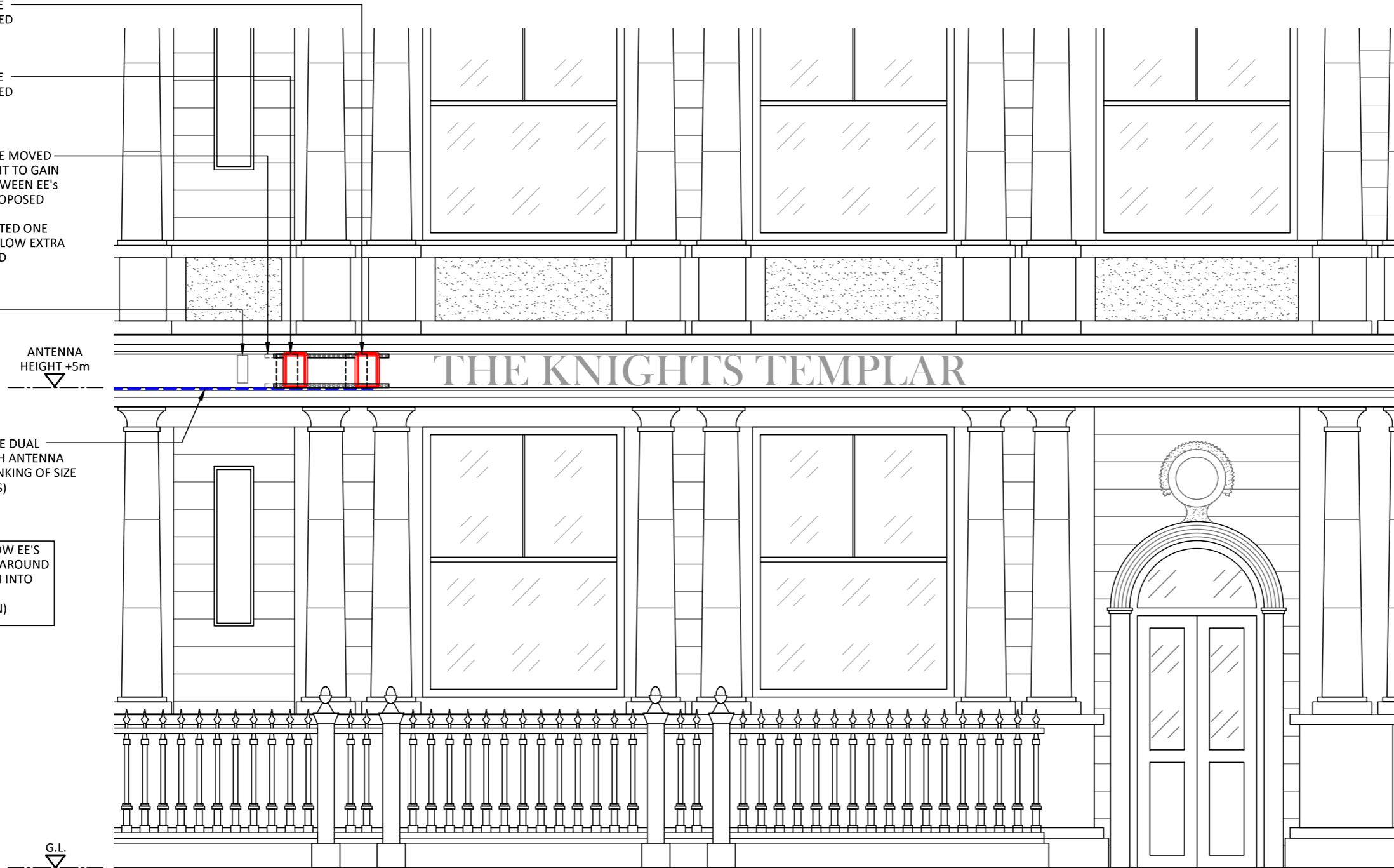
FRONT ELEVATION - PROPOSED ANTENNA LOCATIONS (SCALE 1:50)
