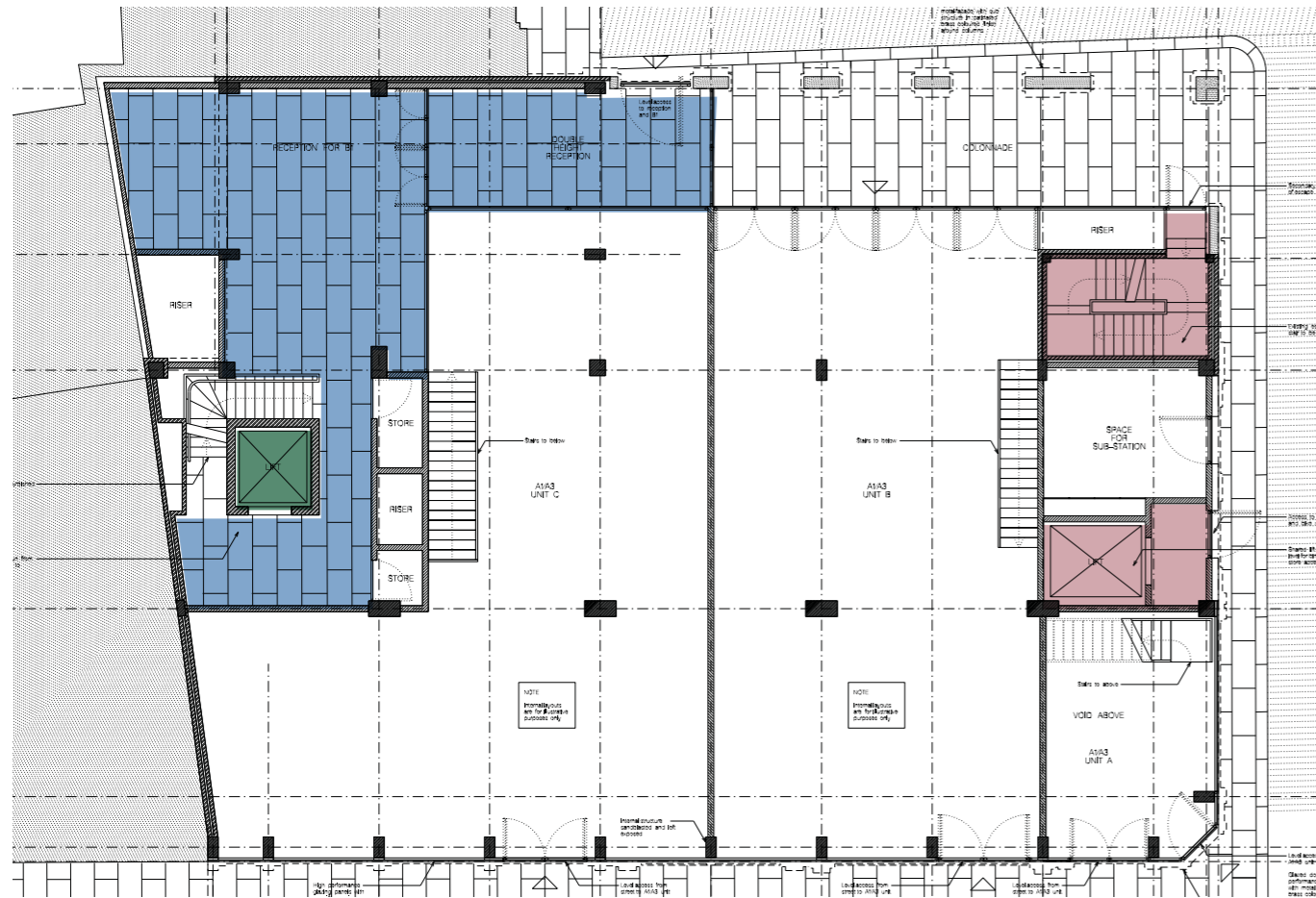
Fig. 183. Ground plan showing single access to office units. Single access to core Lift on key fob Cycle store access on key fob
