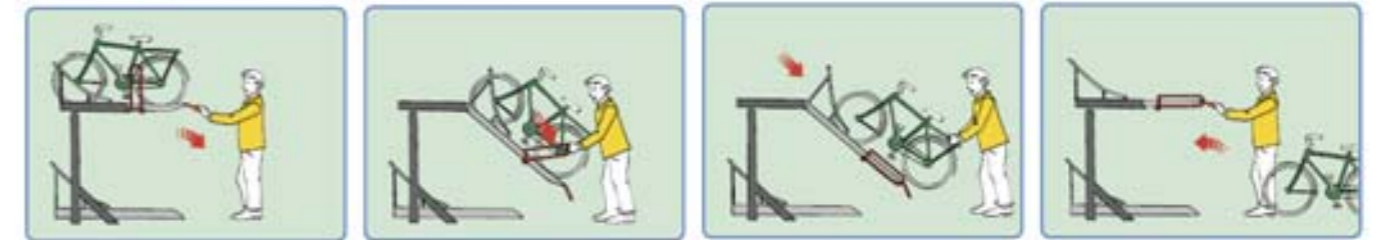
Fig. 178. Josta two tier rack operational instructions.
