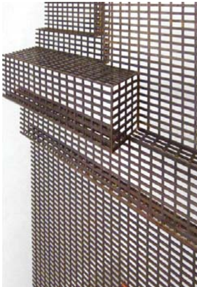
Fig. 73. Perforated brass detail test panel.
