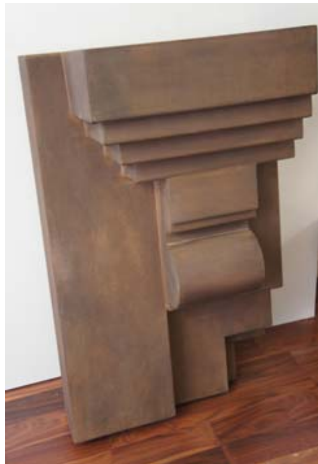
Fig. 74. Solid brass detail test panel.
