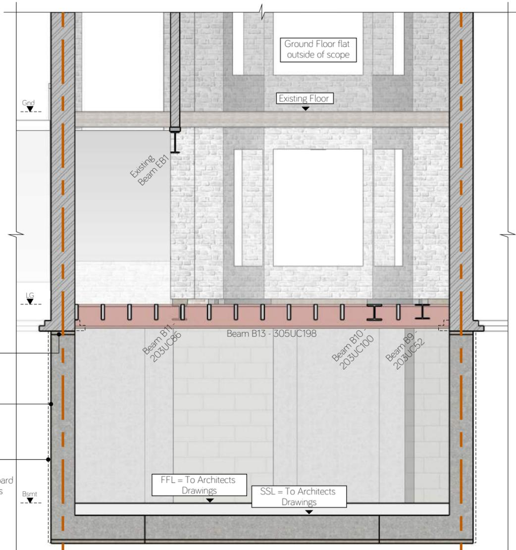
50mm drypack between underpin and underside of existing wall
