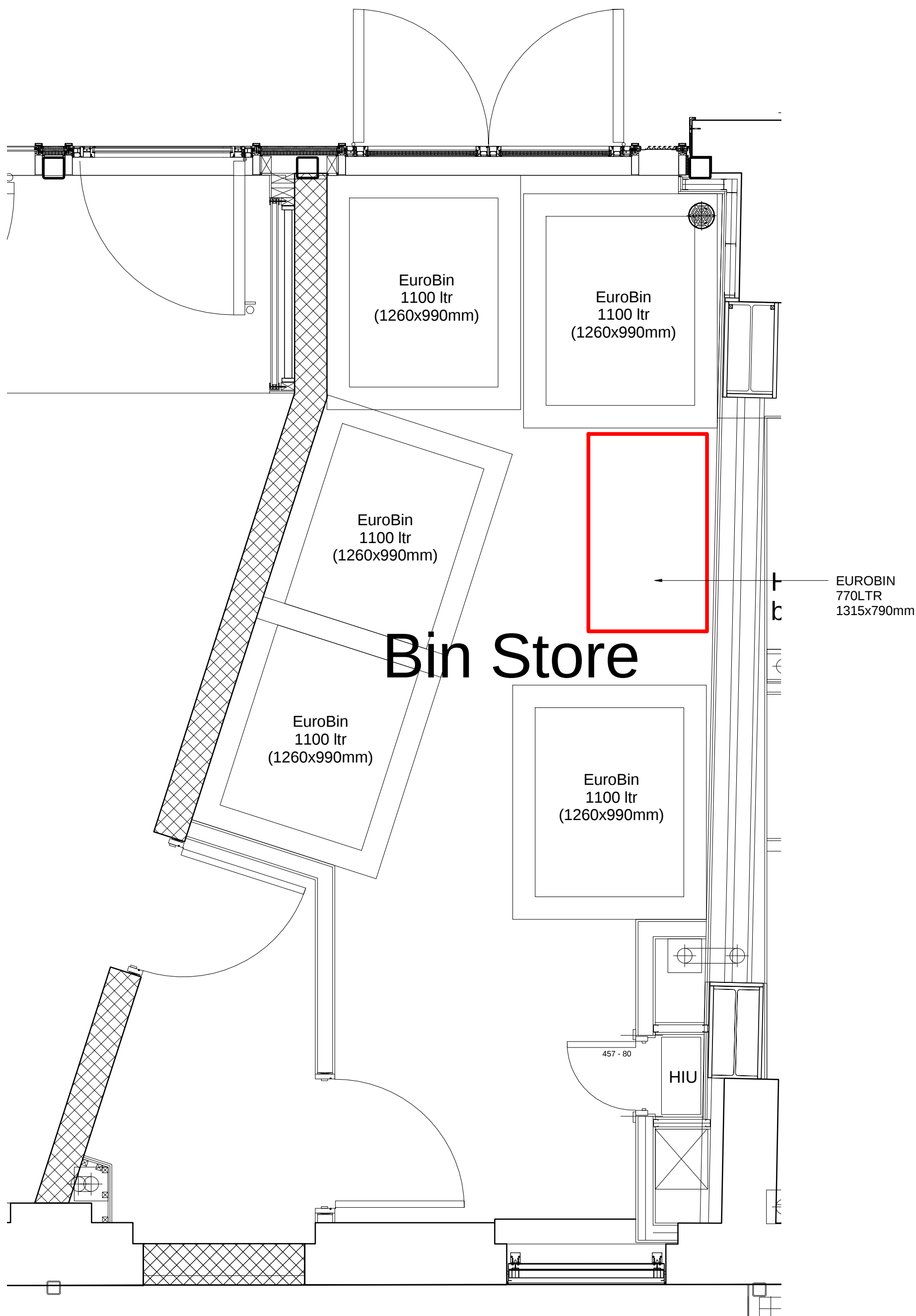
2 PLAN FLOOR PLAN - LEVEL 0 - BIN STORE DETAIL
