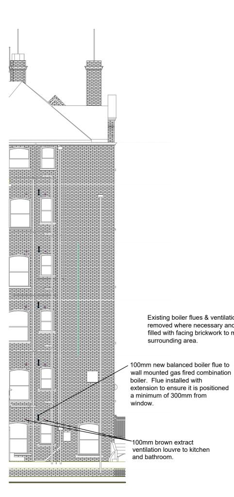
Existing boiler flues & ventilation extracts removed where necessary and apertures filled with facing brickwork to match
