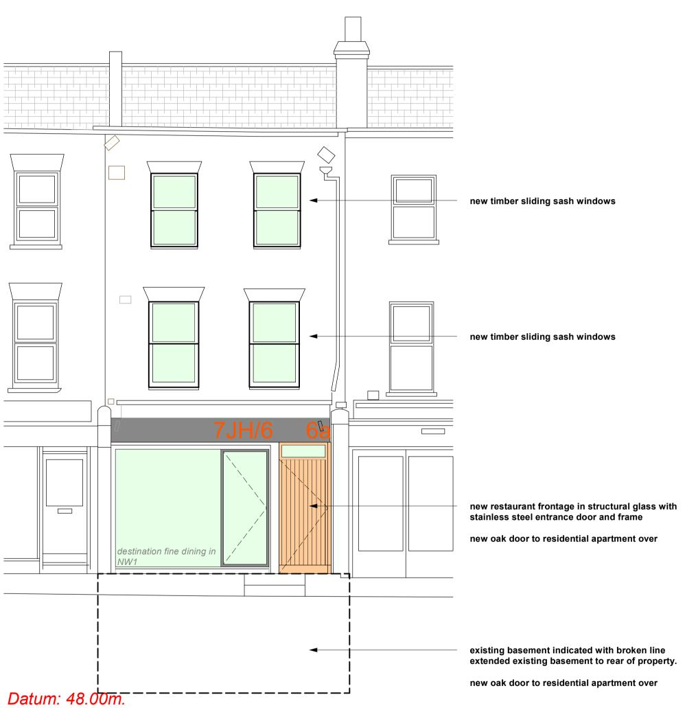
Front Elevation: Proposed scale 1.50 @ A1 (1.100 @ A3)
