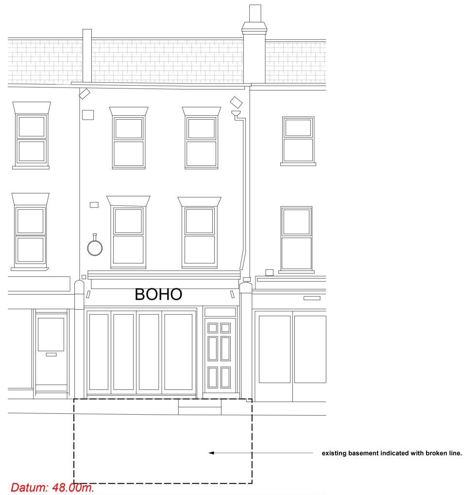
Front Elevation: Existing scale 1.50 @ A1 (1.100 @ A3)
