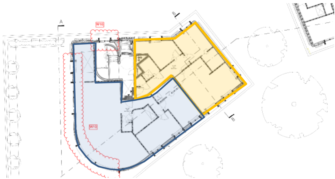
Below: Proposed varied 2 nd floor plan exert (internal layout change only to combine)
