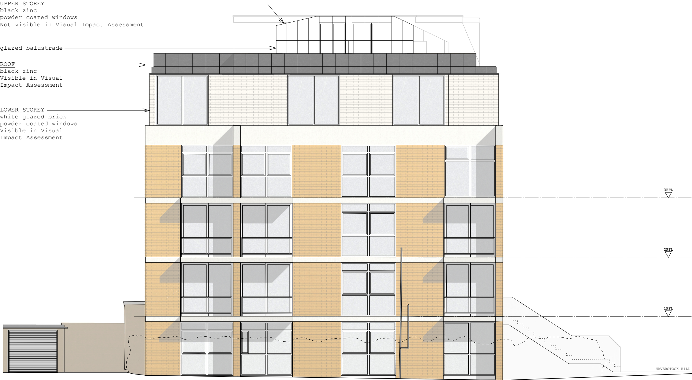
01 Proposed South Elevation
