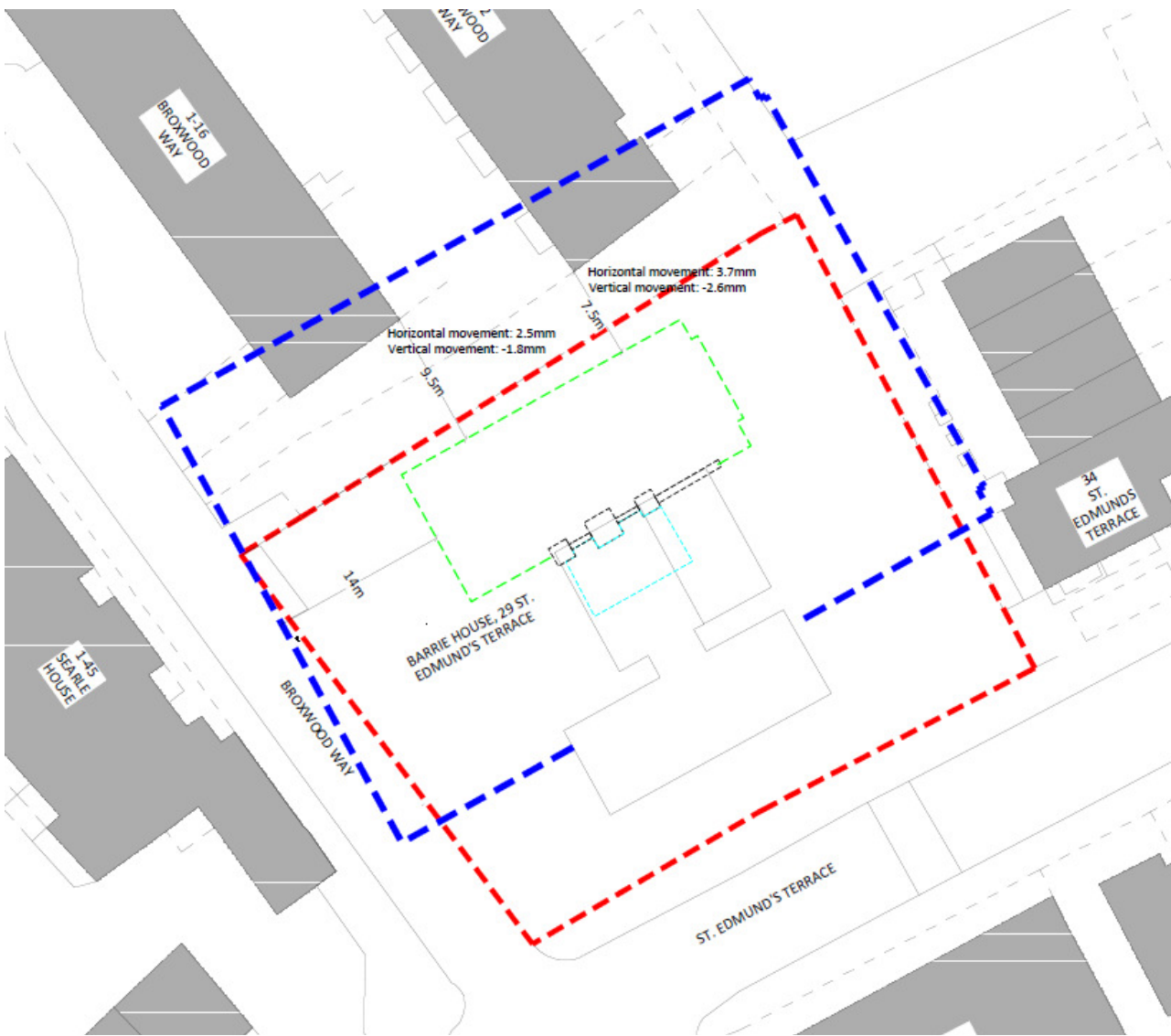
Figure 21 CGL Ground Movement Assessment Summary
