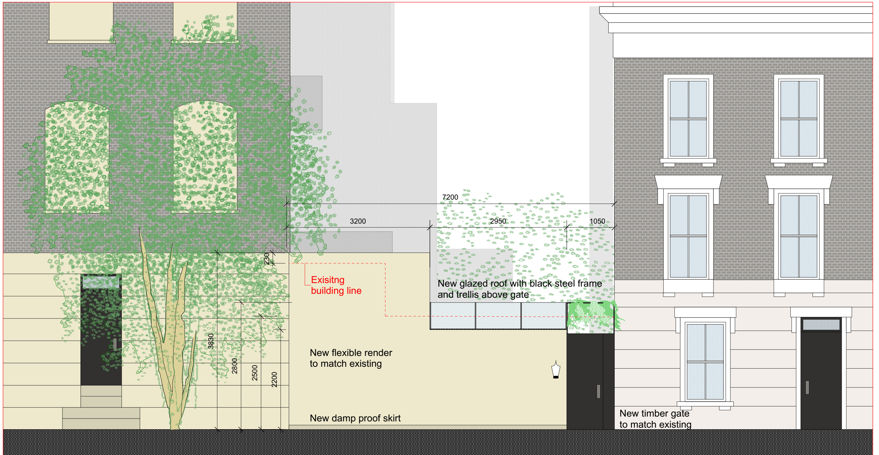
(A/2.21) PROPOSED NORTH ELEVATION: SAINT MARTIN'S LANE scale 1:50
