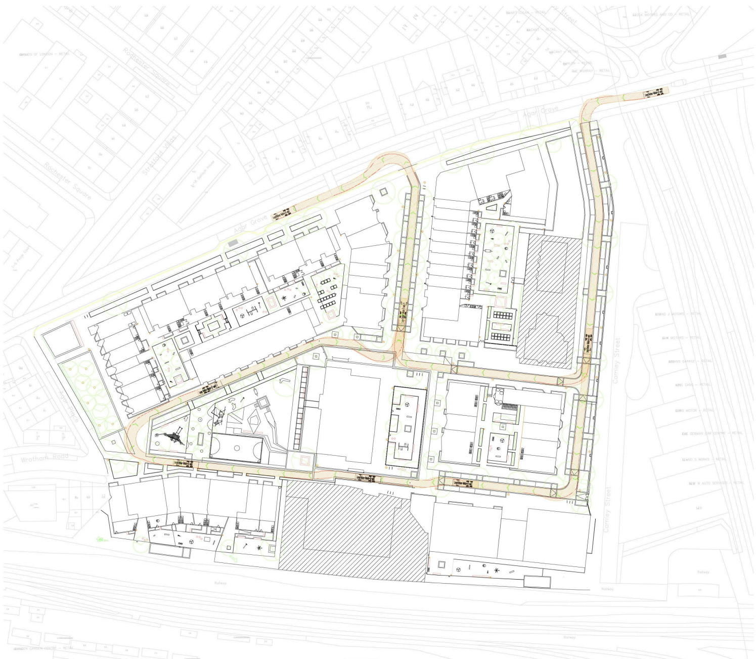
3 Axle Large Refuse Vehicle Swept Path Analysis (NB fire tender would use the same path)
