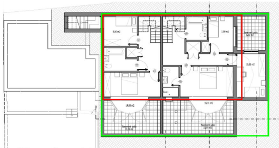
Figure 1.2 Proposed basement plan view, indicating the existing (red) and proposed buildings' footprints
