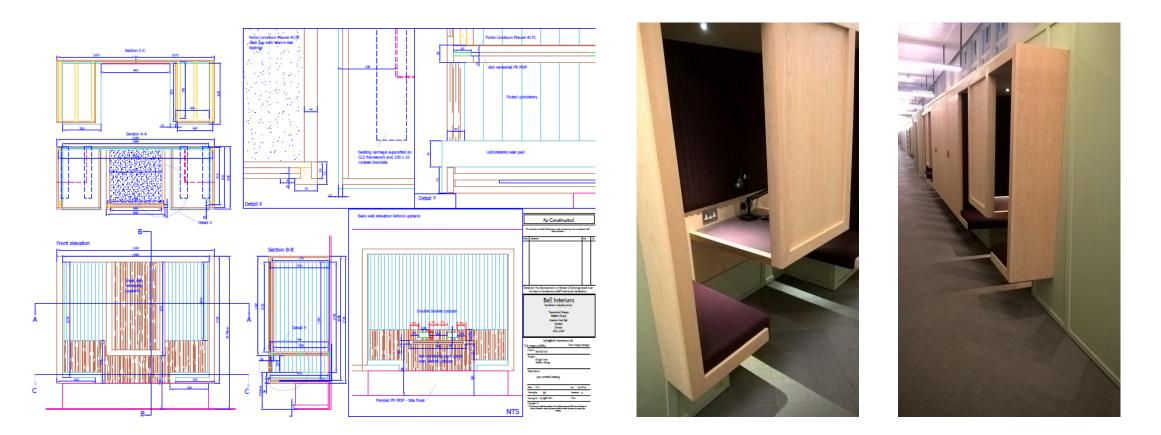
The above shows the detailed plan of the proposed pod, along with photos of existing pods as installed at the south end of the same corridor.
