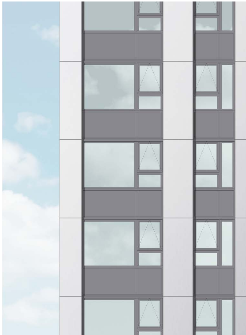
Proposed typical bay elevation in solid aluminium panels (L), as prepared for all three options & presented to the council and residents at the public engagement events (R)
