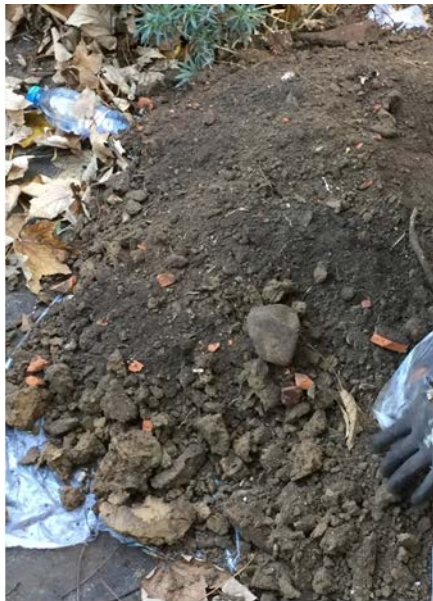
Left: Made Ground observed beneath the rear garden
