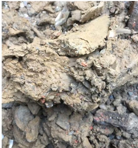
Left: Made Ground observed beneath the rear garden
