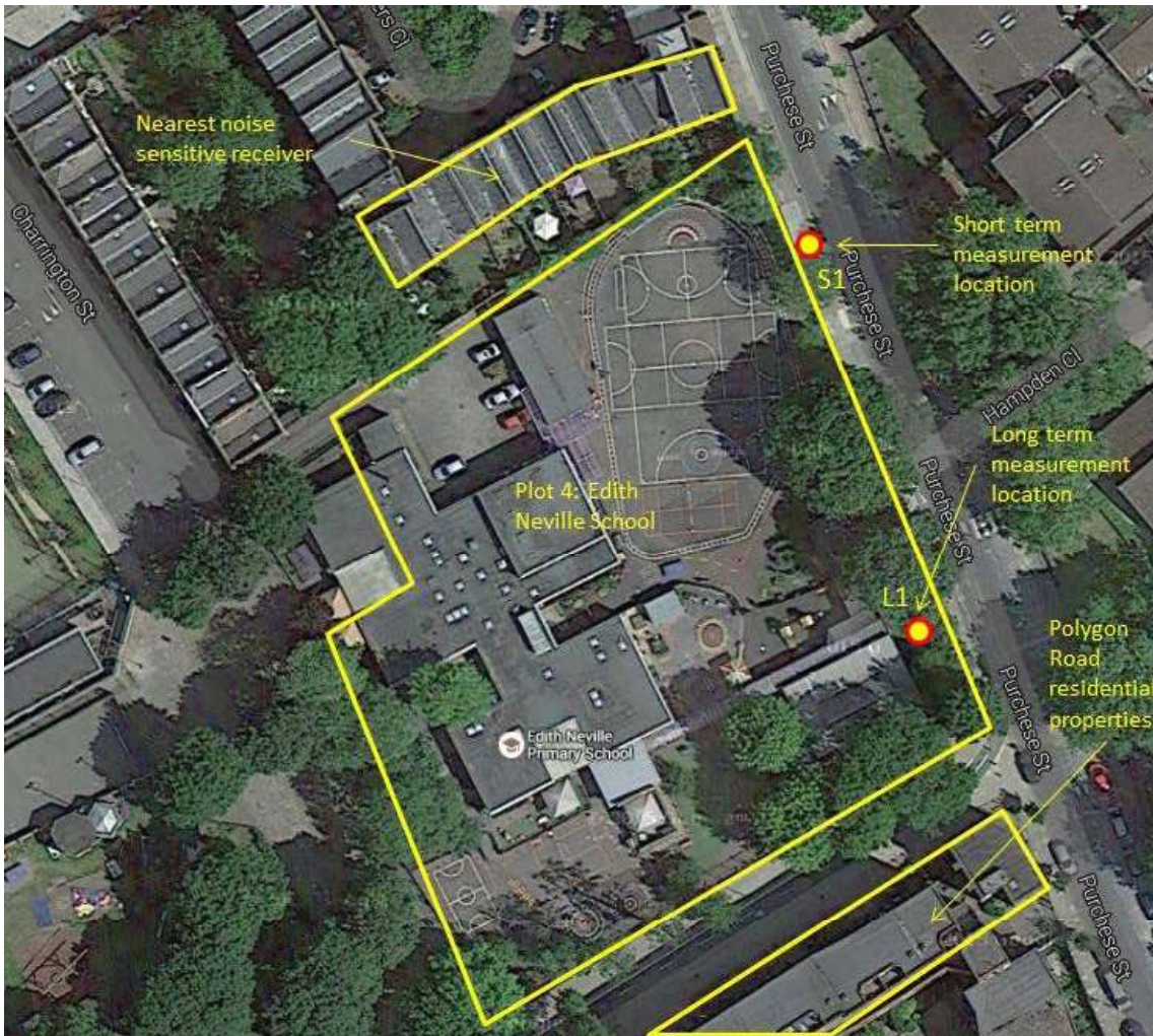
Figure 2: Aerial image of site and noise survey locations
