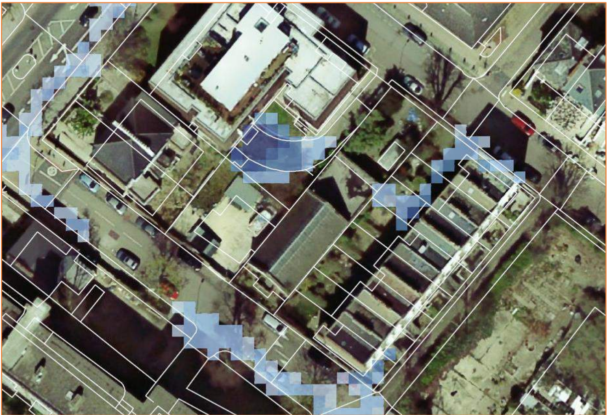
Figure 8: 1:100 year pluvial flood depth mapping (Source: EA)
