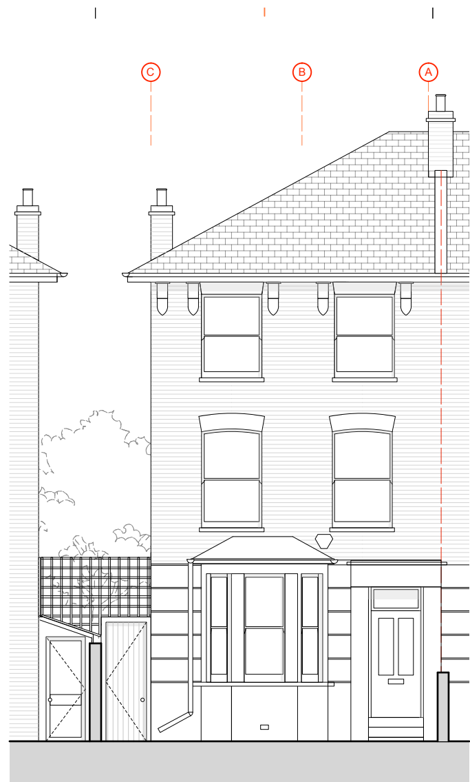
EXISTING FRONT ELEVATION 0 1 2 3 4 5m
