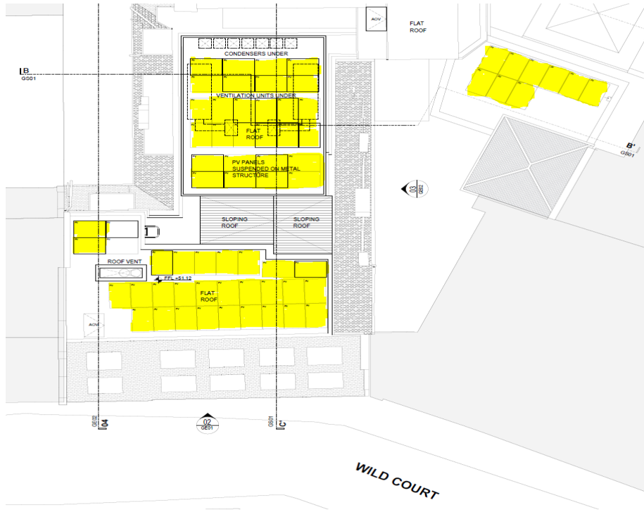
Image shows the propose locations for the PV panels at 8 th floor
