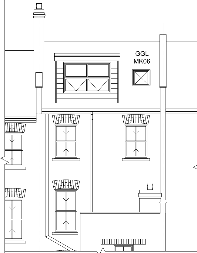
Proposed Southeast (rear) Elevation 1:100
