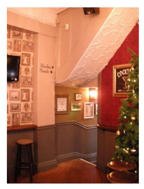
Form a new half glazed fire door above the step line down to the gents toilets. This door will be held open on a magnetic hold linked to the fire alarm.
